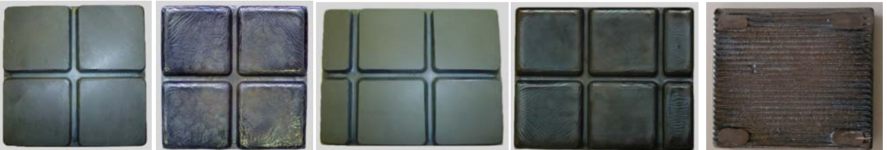
Shown from Left to Right: 8x8 polished, 8x8 as cast, 10x8 polished, 10x8 as cast and back side ribbing.
